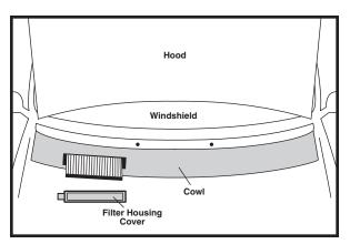
3. Replace filter and reassemble.
